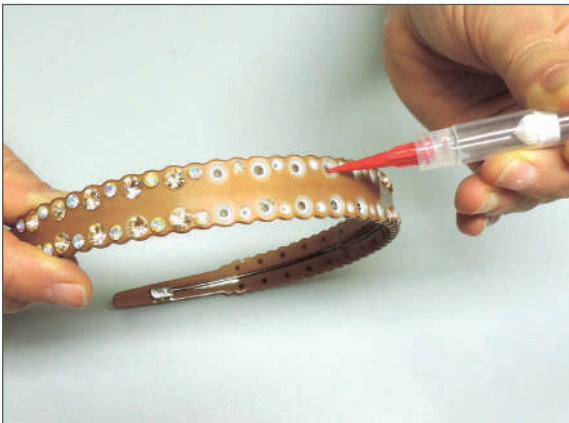
3 A cavity with the glue (applied by hand or with a dispenser).
